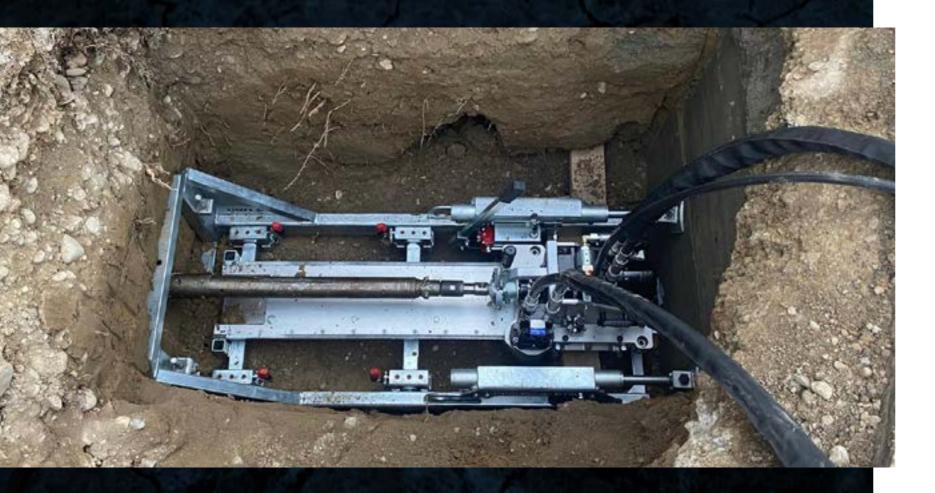
For use in the excavation pit, the MiniRockDrill, including pit frame, can be quickly placed as a complete drilling rig with an excavator. If no lifting gear is available, the pit frame, the drill frame and the rotation gearbox can be installed individually by hand. With the integrated hydraulic hand pump and the two cylinders on the pit frame, a quick fixation is guaranteed and it can be quickly retensioned during operation if the frame becomes unstable.
