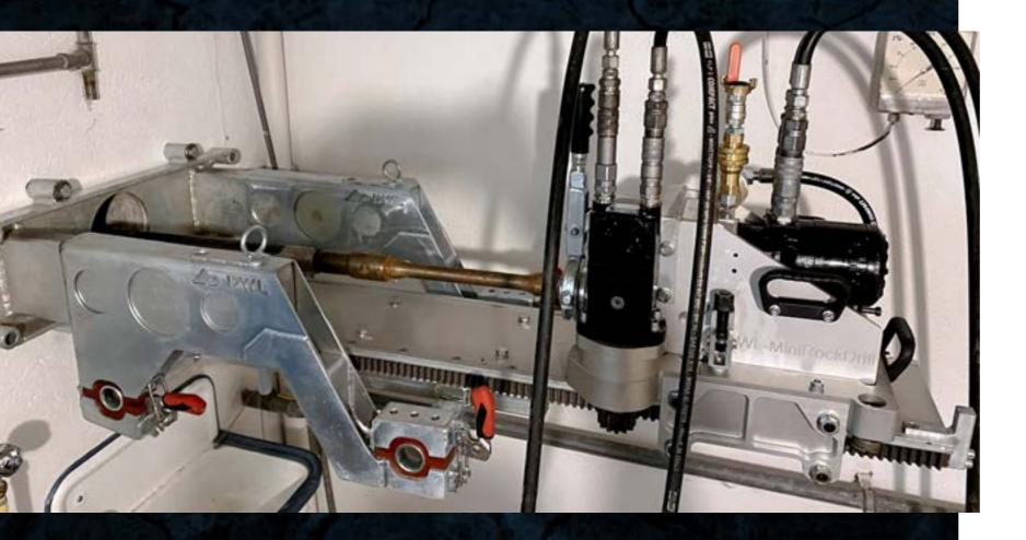
The MiniRockDrill can be easily and quickly placed in the house/cellar/garage to the P2O wall bracket or to a core hole wall bracket. As the unit consists of two main parts, a simple and quick installation is guaranteed, even in confined spaces and with minimum component weights. With our optional DN2OO corehole wall bracket, the installation is even faster directly in the core hole.
